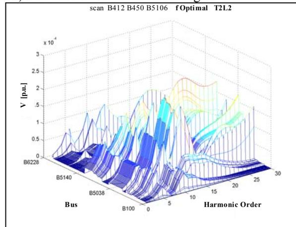
Fig.12 - Voltage frequency response for case T2L2 with optimal filter configuration **fOptimal** and 1∠0° p.u current injection at buses B412, B450 and B5106.
