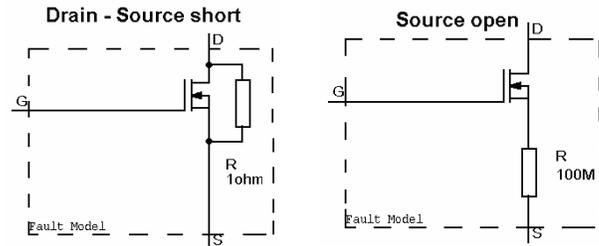
Fig.7. Catastrophic faulty models of nMOS transistor
