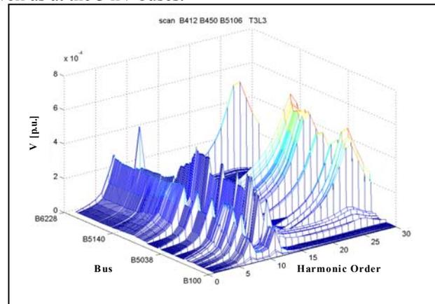
Fig.5 - Voltage frequency response for case T3L3
