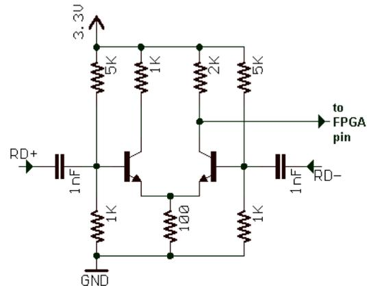
Fig. 4. Differential circuit for reception
