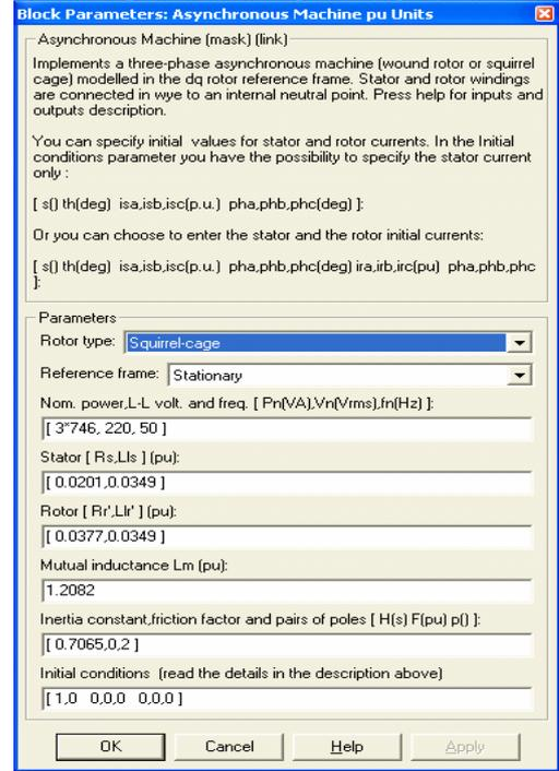
Fig. 6. The parameters of the induction motors.
