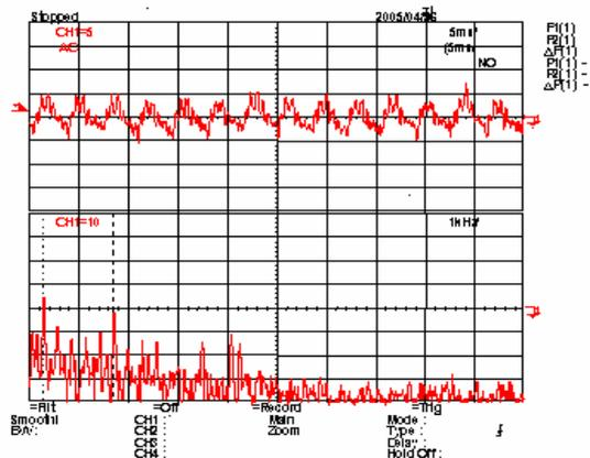
Figure 14. Output voltage ripple and its frequency spectrum at full power
