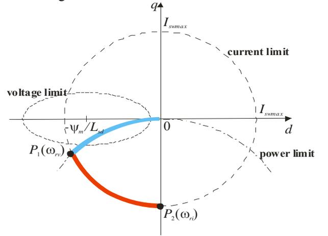
Fig. 1 Trajectory of stator current space vector during braking
