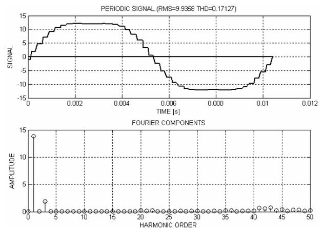
Fig. 10. Inverter output pole voltage and harmonic analysis in inverter discrete model. Switching elements voltage drops are not considered
