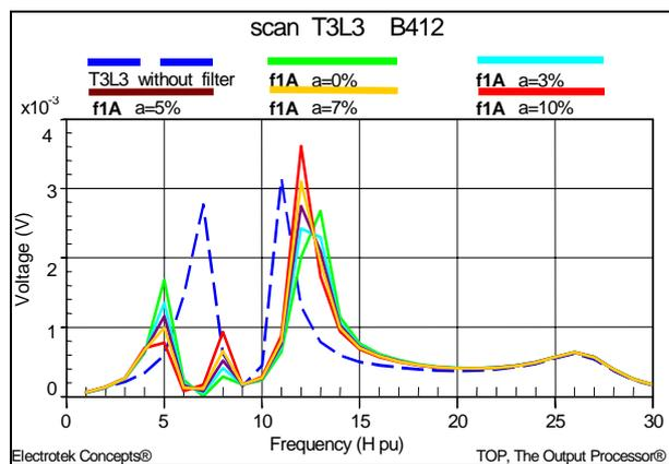
Fig.6 - Impact of tuning factor on frequency response of bus B412
