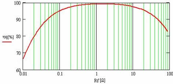
Fig. 11. Efficiency vs. output resistance calculated using ANSYS
