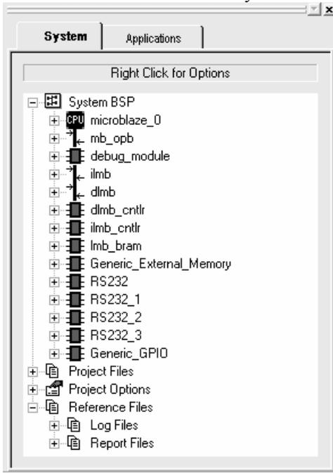
Fig. 3. SoC Structure (Xilinx EDK)
