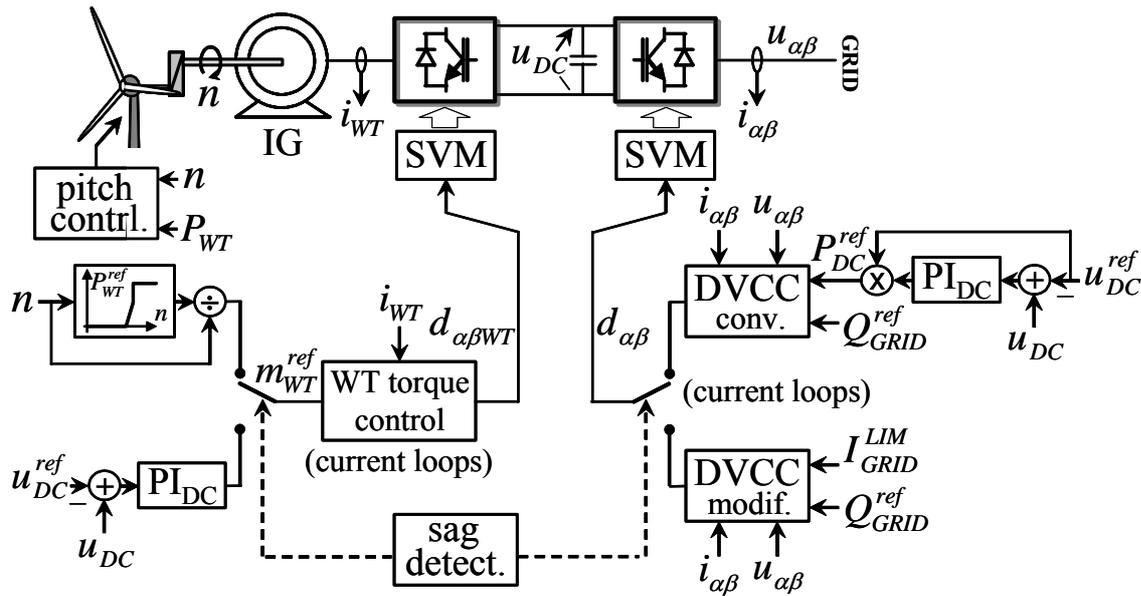
Fig. 5. WT control structure
