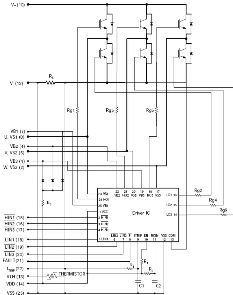
Fig. 6: Internal schematics of IRAMS Intelligent Power Module.
