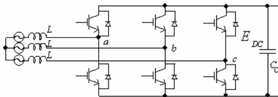
Fig. 4. Regenerative front-end converter
