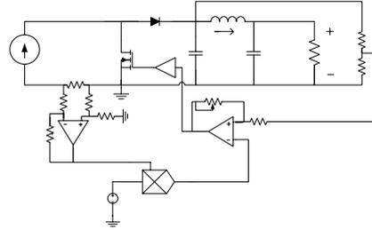
Fig. 7 Practical implementation of a BOF converter-based R-yrator
