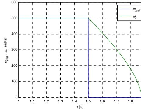
Fig. 3 Reference and actual motor speed during braking
