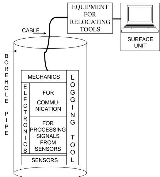
Fig. 1. A block diagram of a system for boreholes investigation.
