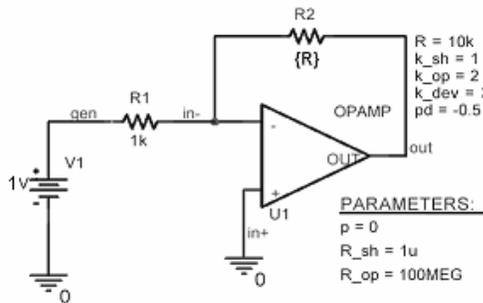
Fig. 2. DC Amplifier with a faulty model for  $R_2$ .
