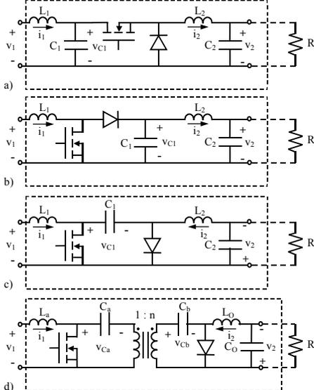
Fig. 2 Fourth order converters with non-pulsating input and output currents a) buck converter with input filter b) boost converter with output filter c) Čuk converter d) Čuk converter with galvanic isolation
