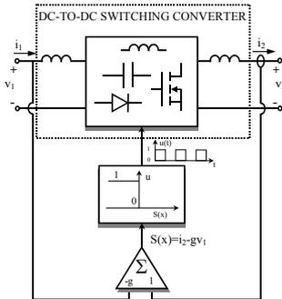
Fig. 1 Block diagram of a dc-to-dc switching regulator with gyrator characteristics
