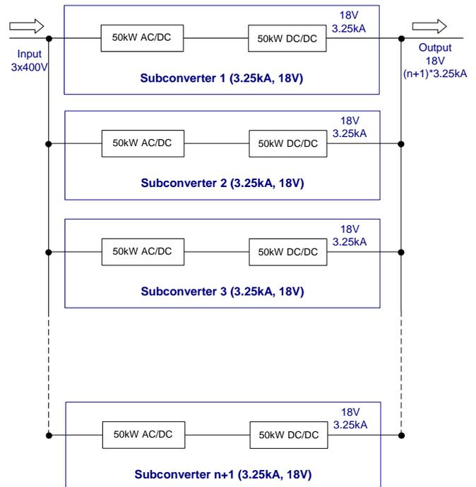
Figure 8. n+1 redundancy concept
