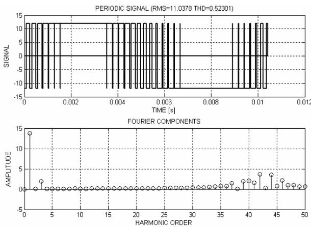
Fig. 7. Inverter output pole voltage and harmonic analysis in inverter pulse model. Switching elements voltage drops are not considered
