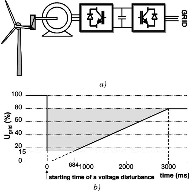
Fig. 1. a) Wind turbine with fully- controlled IG; b) E.ON requirements for a WT grid connection
