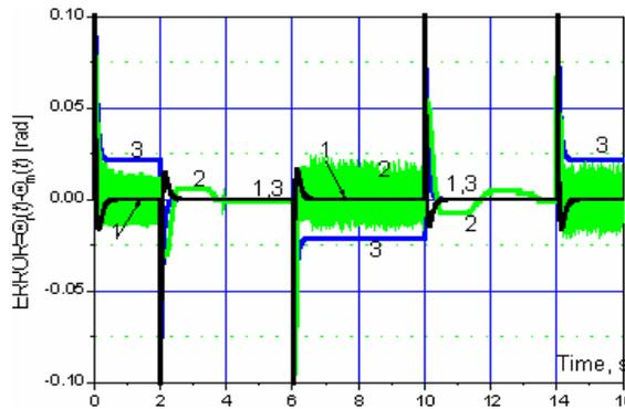
Fig. 3. Tracking error of the referent position profile (Fig. 2): the proposed system ( $\rho=0.5$ ,  $h=16$ ): 1- simulation, 2-experiment, 3-the Golo's system (simulation).
