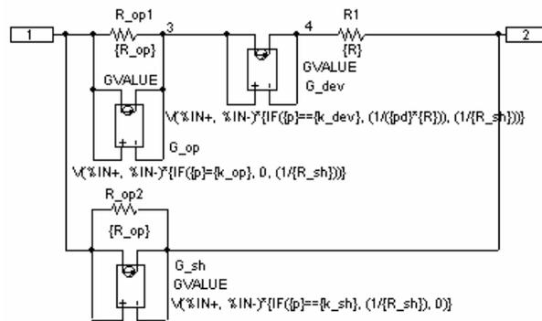
Fig. 1. Schematic diagram of the resistor faulty model
