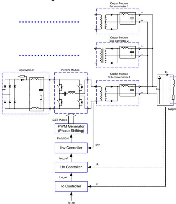
Figure 5. Control structure
