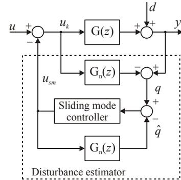
Fig. 1. Structure of DSMC based disturbance estimator.
