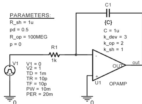
Fig. 5. Integrator with faulty model of  $C$
