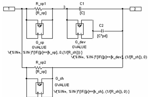
Fig. 4. Schematic diagram of the capacitor's faulty model
