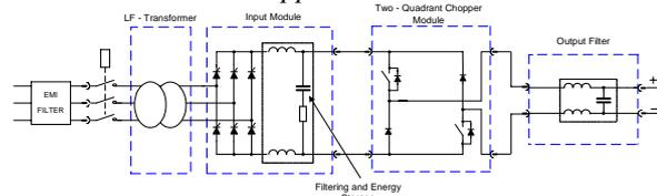
Figure 4. Energy recovery pulsed PSU with 2-quadrant chopper module
