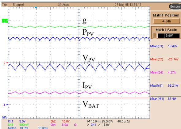
Fig. 14 Steady-state waveforms of a Cuk converter-based G-yrator with controlled input current supplying 24 V battery.
