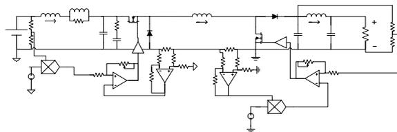
Fig. 8 Practical implementation of the cascade connection of a buck converter with input filter G-yrator and a boost converter with output filter R-yrator.
