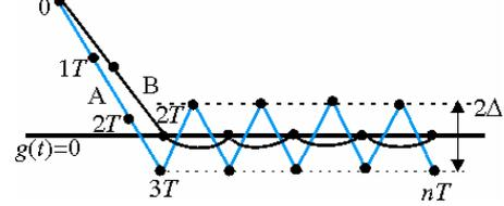
Fig. 1. Two basic types of discrete-time sliding mode:
