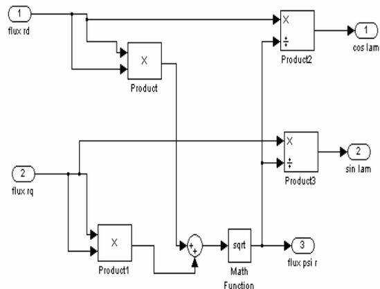
Fig. 4. The phasor analyzer AF– unfolded scheme.
