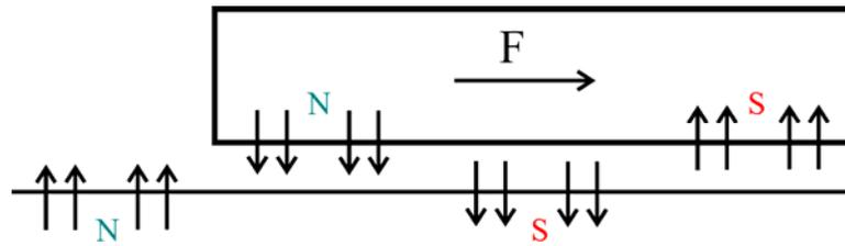
Fig. 12: Linear electrical actuator – principles of operation.
