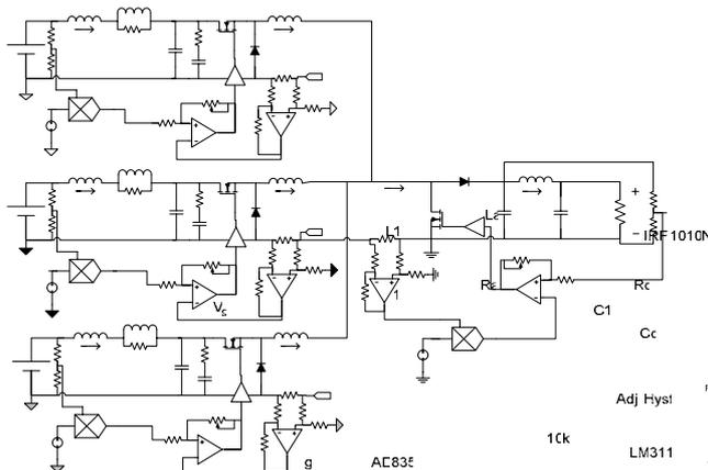
Fig. 9 Practical implementation of a cascade connection of 3 paralleled power G-yrators and a power R-yrator
