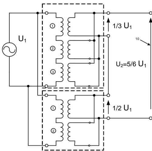
Fig. 3. Example of modular transformer with  $k=1,2$  ( $m=2$ ,  $n_1=3$ ,  $n_2=2$ )
