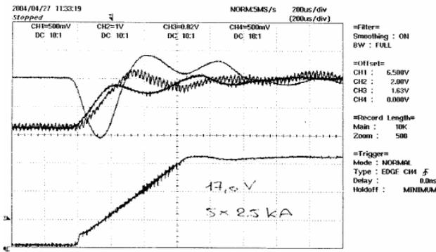
Figure 11. Magnet voltage and sub-converter current when one sub-converter fails (time trace 200µs/div)
