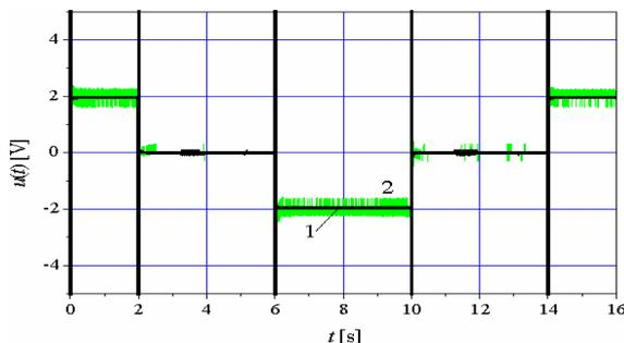
Fig. 5. Control signal of the proposed system for tracking the referent profile (Fig. 2): 1 - simulation; 2 - experiment.
