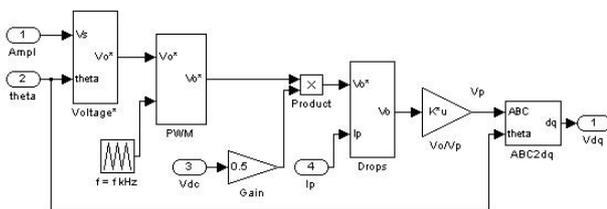
Fig. 4. Scheme of pulse model of inverter
