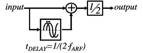
Fig. 3. Control diagram of ARF
