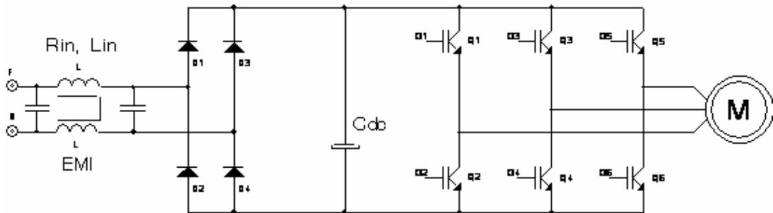
Fig. 7: Single-phase supplied inverter with the 3-phase output.
