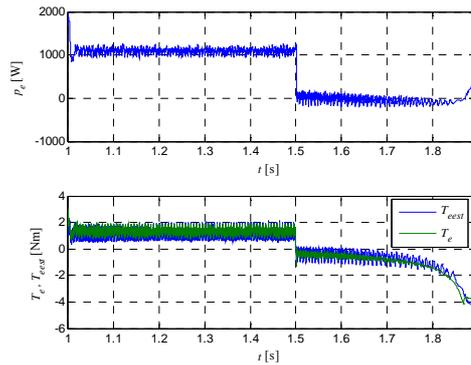
Fig. 6 Motor electrical power and electromagnetic torque during braking
