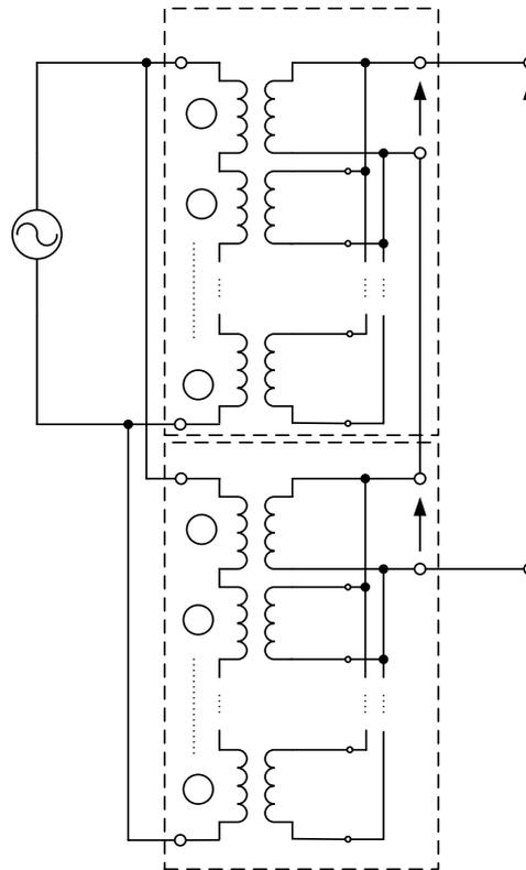
Fig. 2. Example of modular transformer with ( $m=2$ , with any  $n_1, n_2$ )
