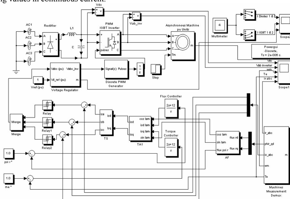
Fig. 1. The adjusting scheme of the induction motor torque supplied through a voltage-regulated inverter with direct measure of the field and with rotor flux orientation.
