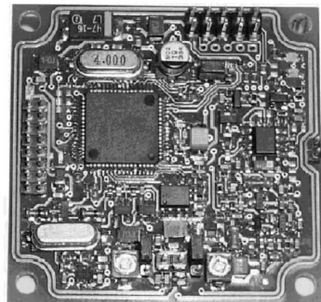
Fig. 2. ID.ISC.M02 RFID Reader
