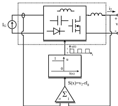
Fig. 6 Block diagram of a dc-to-dc switching regulator operating in sliding-mode with R-yrator characteristics
