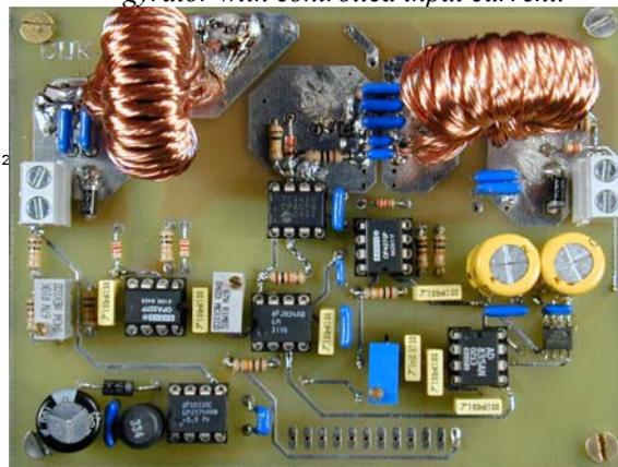
Fig. 12 A 7.5mW Cuk converter-based G-yrator with controlled input current.
