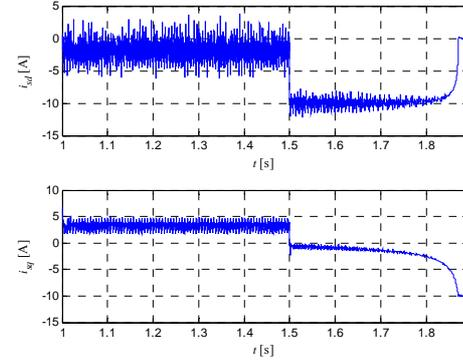
Fig. 4 Stator d and q-axis currents during braking
