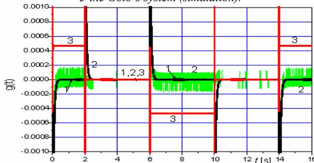
Fig. 4. Switching function dynamics in tracking of the referent position profile (Fig. 2): the proposed system: 1 - simulation; 2 - experiment; 3-the Golo's system (simulation).
