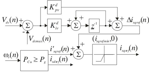
Fig. 2 Block-diagram of braking control system
