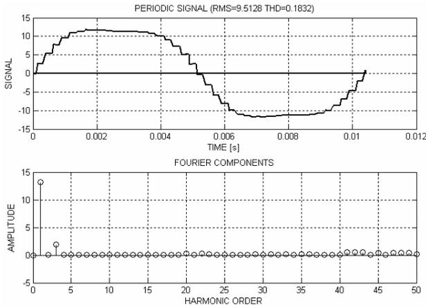
Fig. 11. Inverter output pole voltage and harmonic analysis in inverter discrete model. Switching elements voltage drops are considered
