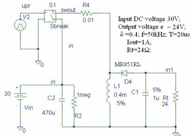
Fig. 11. A DC-DC converter, the scheme under test
