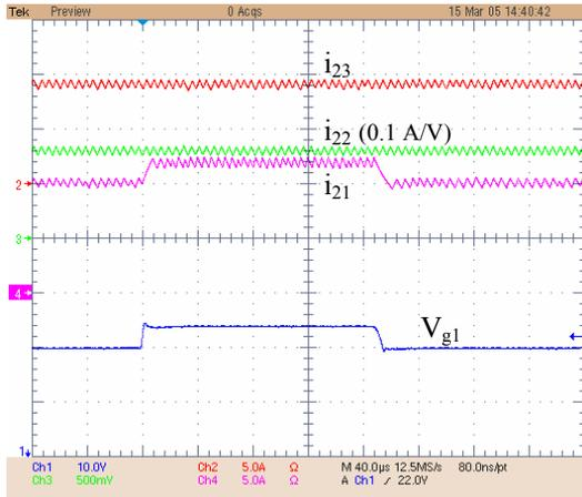
Fig. 5 Experimental behaviour of 3 paralleled BIF converter-based G-yrators to a pulsating input voltage in gyrator #1.
