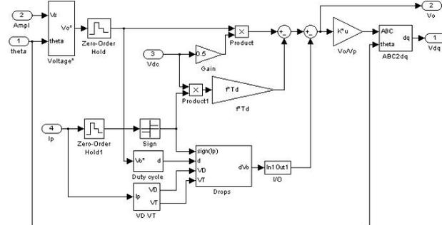
Fig. 5. Scheme of discrete model of inverter
