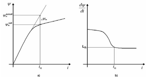
Fig. 3. Magnetizing curve (a) and its derivation by magnetizing current (b)
