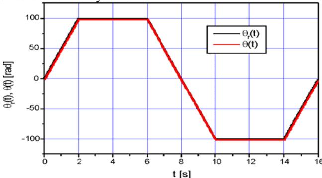
Fig. 2. Referent position profile  $\theta_r(t)$  and obtained motor shaft position  $\theta(t)$  using the proposed control.
