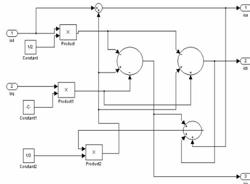
Fig. 3. The block of the transformation of the bi-phase system in three-phase system of measures – unfolded scheme
