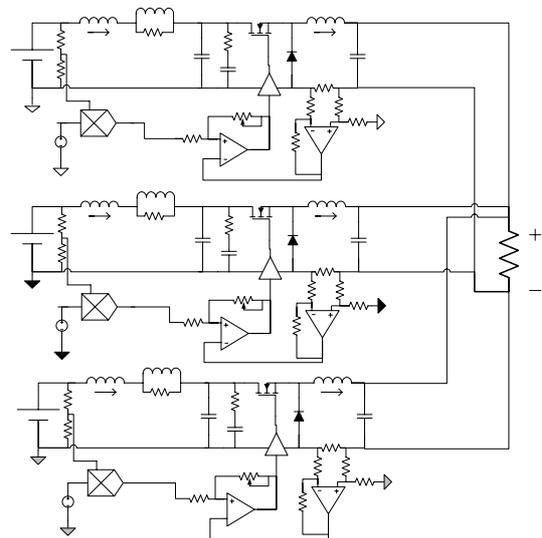
Fig. 4 Practical implementation of the parallel connection of three Buck converters with input filter G-yrators.
