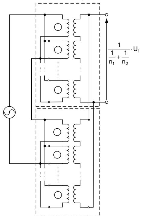
Fig. 5. Scheme diagram of two  $n$ -modules<sup>-1</sup> transformers
