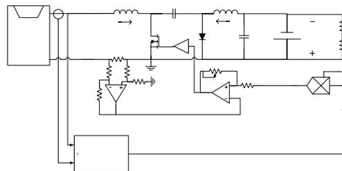
Fig. 13 Cuk converter-based G-yrator with controlled input current with MPPT function
