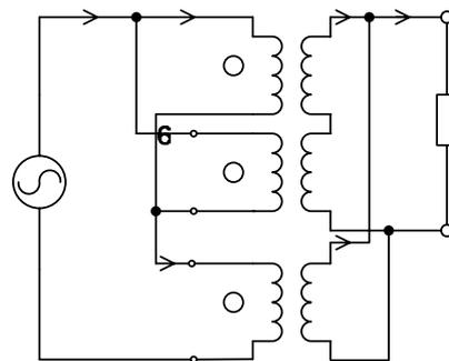
Fig. 10. Scheme of winding configuration in experimental transformer
