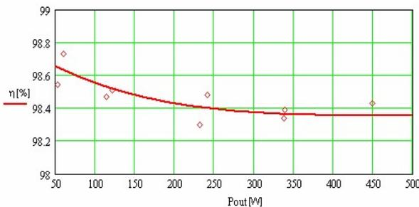
Fig. 12. Efficiency vs. output power of experimental transformer
