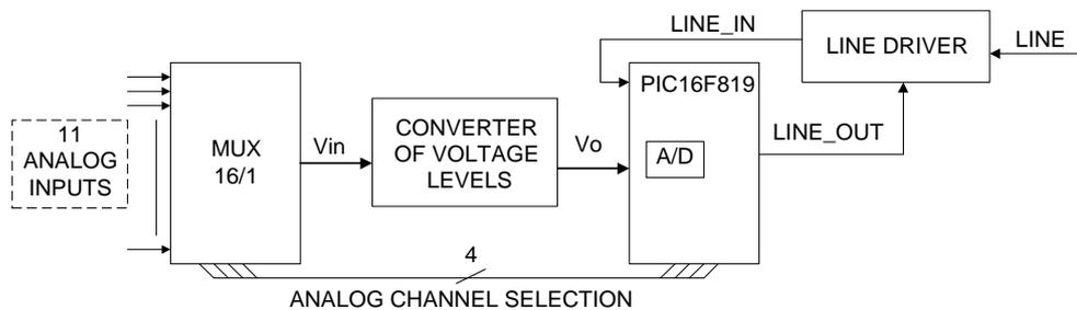
Fig.4. The block diagram of the connection between the universal A/D converter protocol device and a line driver.
