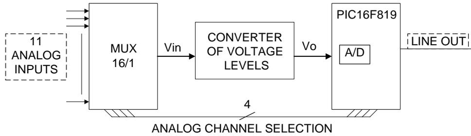
Fig.2. A block diagram of the universal A/D converter protocol device
