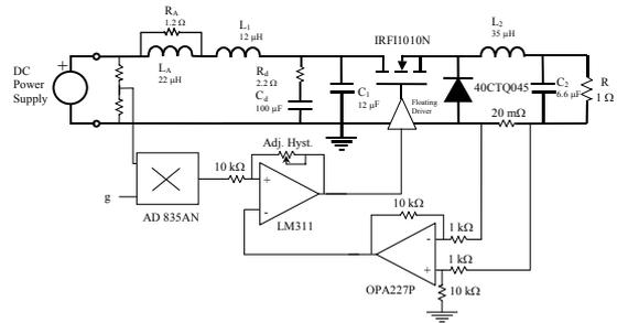
Fig. 3 Practical implementation of a BIF converter-based gyrator  $L_1=12 \mu H$ ,  $L_2=35 \mu H$ ,  $C_1=12 \mu F$ ,  $C_2=6.6 \mu F$ ,  $C_d=100 \mu F$ ,  $R_d=2.2 \Omega$ ,  $L_a=22 \mu H$ ,  $R_a=1.2 \Omega$ ,  $g=0.5 \Omega^{-1}$ ,  $R=1 \Omega$
