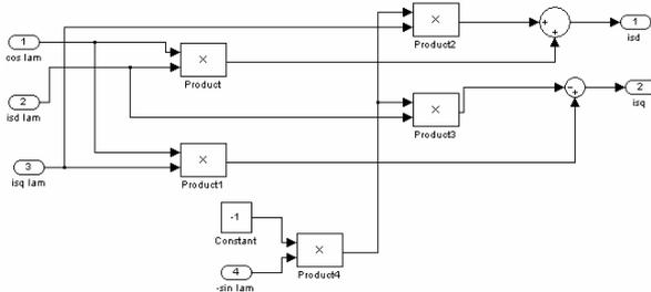
Fig. 5. The axes transformation block TA1– unfolded scheme.
