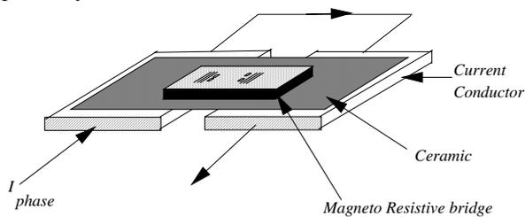
Fig. 10: Usage of magnetoresistive bridge in current sensing
