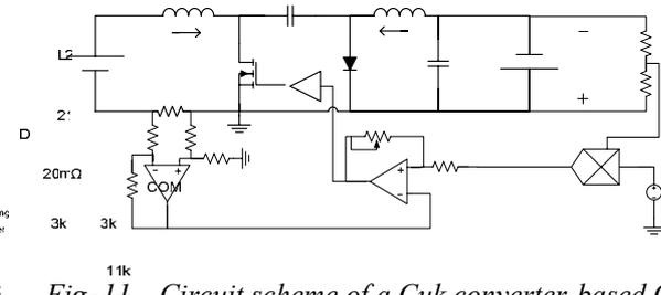
Fig. 11 Circuit scheme of a Cuk converter-based G-yrator with controlled input current.
