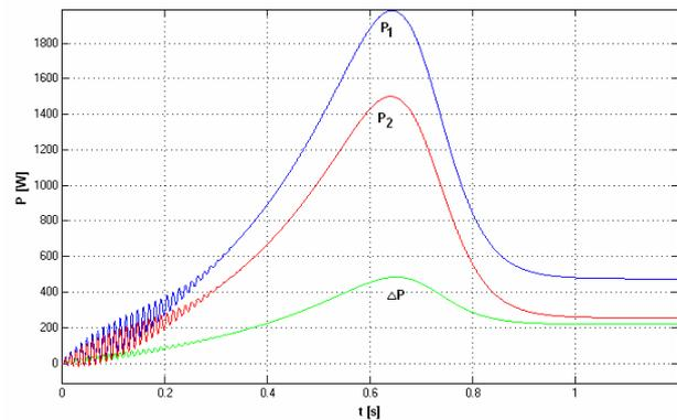
Fig. 14. Input and output power and total losses course in drive mechanical part during vehicle start
