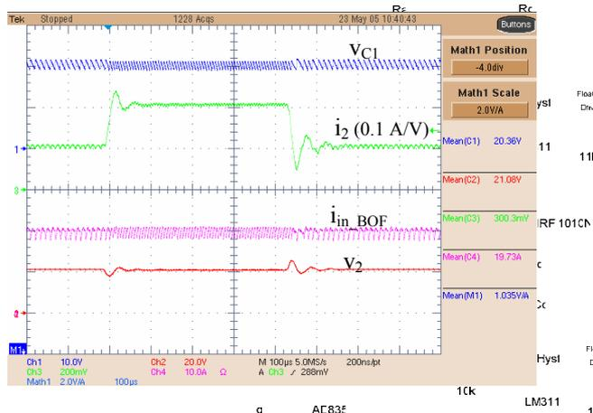
Fig. 10 Experimental response of the circuit of Fig. 9 to load variations of step type
