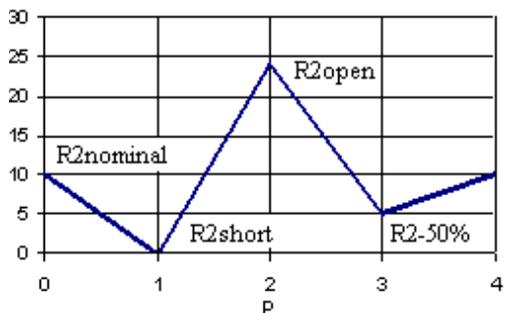
Fig.3. Values of  $V(out)$  versus the fault number  $p$
