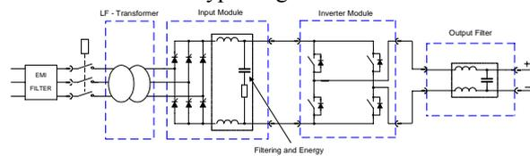
Figure 3. Bipolar pulsed PSU with inverter / 4-quadrant chopper module
