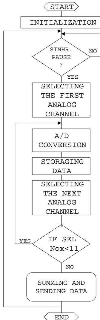
Fig. 5. The algorithm for the PIC 16F819.
