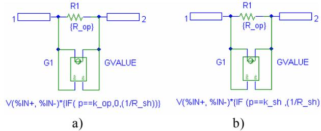
Fig. 8. Faulty model of an "open" circuit(a) and of a "short" circuit (b)
