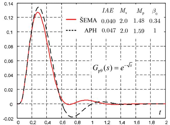
Fig. 11. Load disturbance response for  $G_{p9}(s)$
