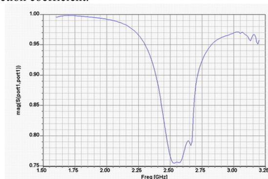
Fig.9. Magnitude of the reflection coefficient
