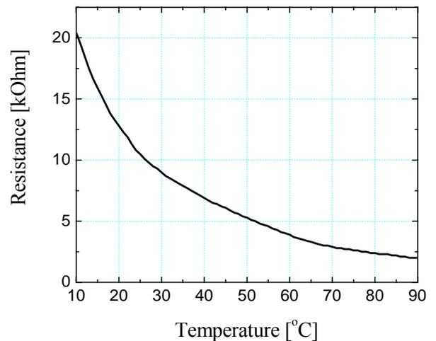
Fig.4. Resistance-temperature calibration curve
