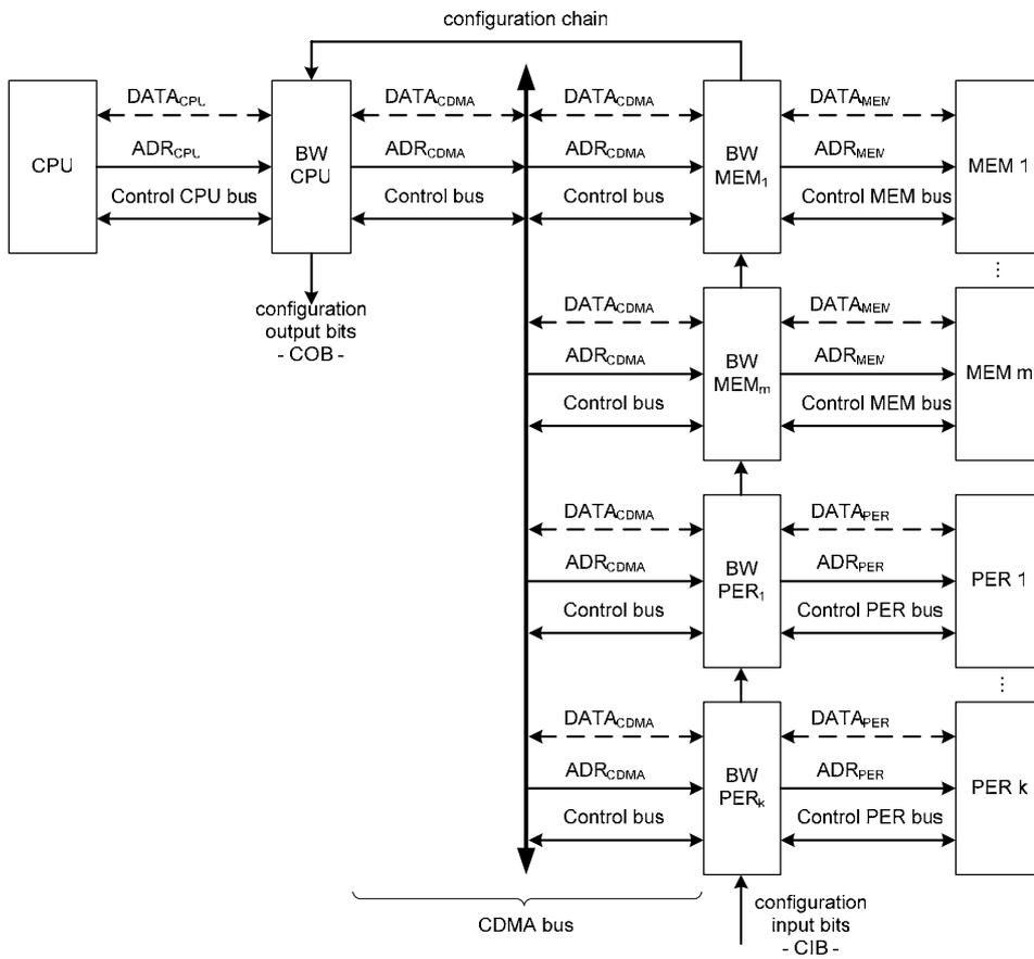
Fig.3. Uni-processor 32-bit system organized around system bus which uses wrappers as interface logic and CDMA transmission technique for data transfer
