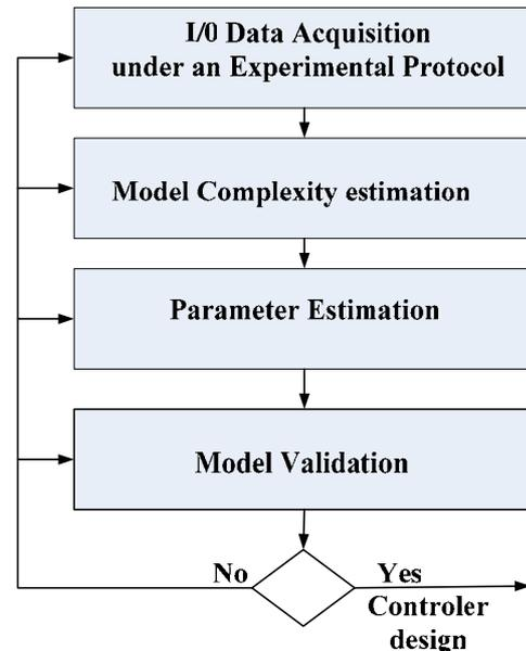
Fig.1. Iterative dynamic systems identification process and parameters estimation
