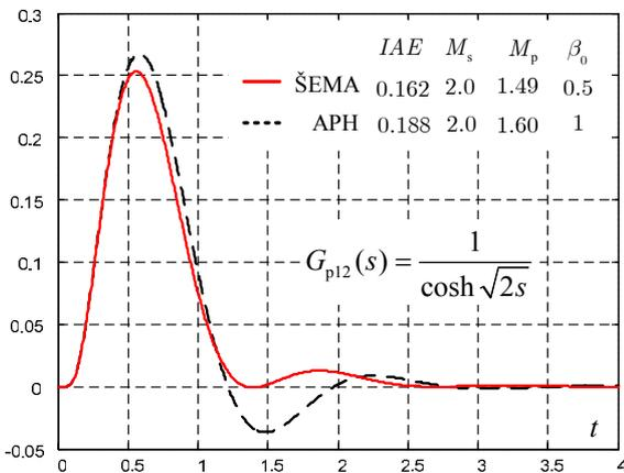
Fig. 14. Load disturbance response for  $G_{p12}(s)$ Table 1. Parameters of the optimally tuned PI controller obtained by applying the combined criterion  $J_c$ , for  $G_{pn}$ ,  $n=1,2,\dots,12$ .
