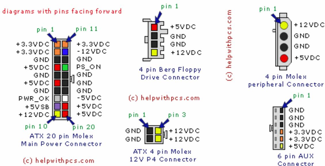
Fig.1. Arrangement of pins for connectors of ATX supply
