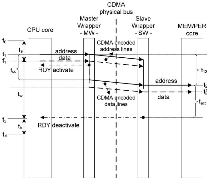
Fig.6. Signaling scenario of a Write processor cycle
