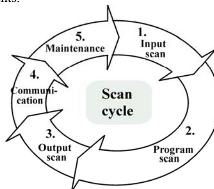
Fig.3. Scan Cycle ( Typical values for an Allen-Bradley Micrologix controller: input/output scan time of 8 $\mu$ s; housekeeping 180 $\mu$ s )
