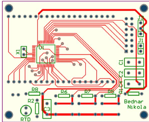
Fig.6. Bottom view of the PCB
