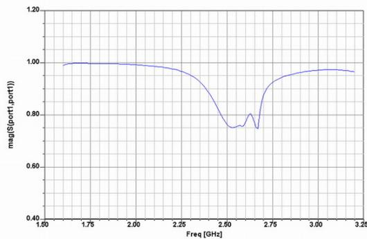
Fig.10. Magnitude of the refl. coeff. in case the separation between the substrate and the end of the waveguide is 5 mm
