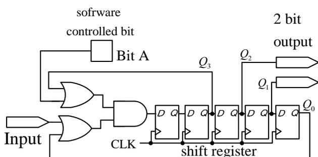
Fig.1. Hardware schematic for binary signal processing.
