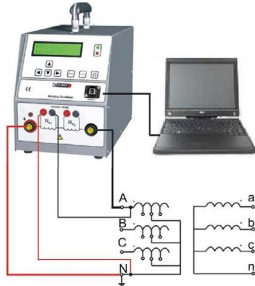
Fig.5. Method for the OLTC analysis of power transformers
