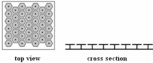
Fig.4. A mushroom structure with hexagonal metal plates
