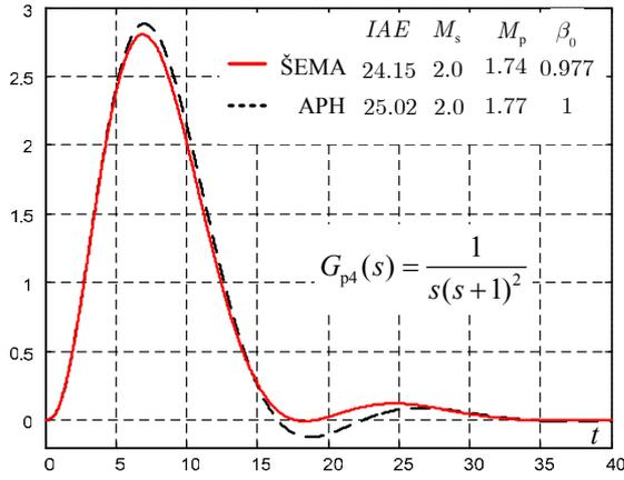
Fig. 6. Load disturbance response for  $G_{p4}(s)$
