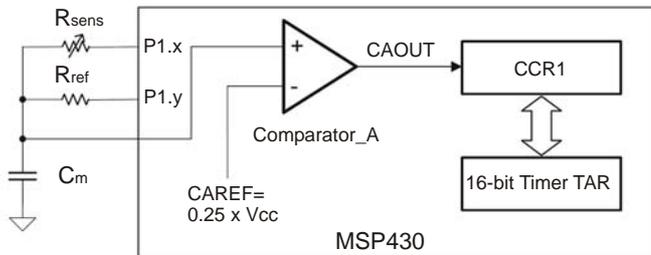
Fig.2. The principle of resistance measurement
