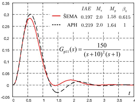
Fig. 13. Load disturbance response for  $G_{p11}(s)$
