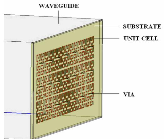
Fig.13. The structure with vias between the unit cells and the ground layer
