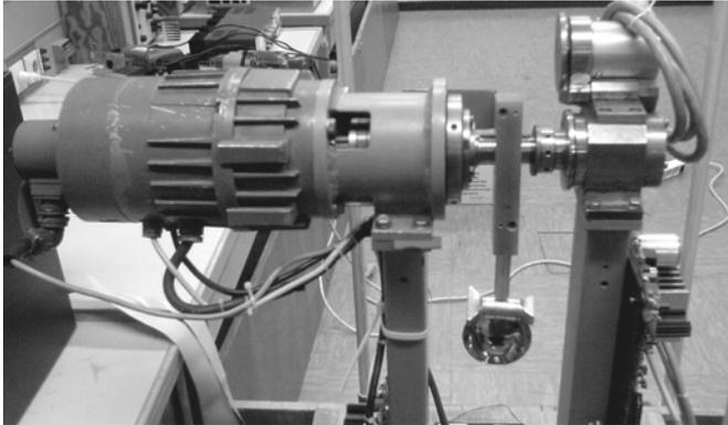
Fig.2. Apparatus for motor control of human arm in ballistic tasks of target hitting exercise
