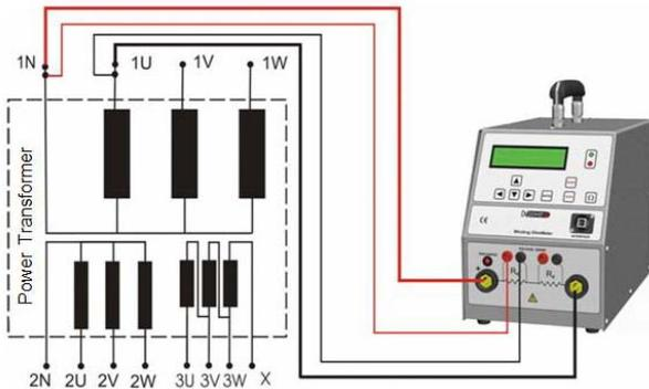
Fig.3. Method for winding resistance measurement of power transformer
