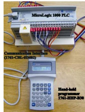
Fig.6. A hand-held PLC programmer linked with controller
