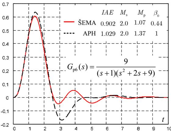
Fig. 8. Load disturbance response for  $G_{p6}(s)$
