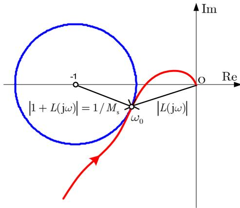
Fig.2.  $M_s$  circle and Nyquist curve  $L(j\omega)$  of the optimally tuned closed-loop system. At the frequency  $\omega_0$  the sensitivity has its largest value  $|S(j\omega_0)| = M_s$ .
