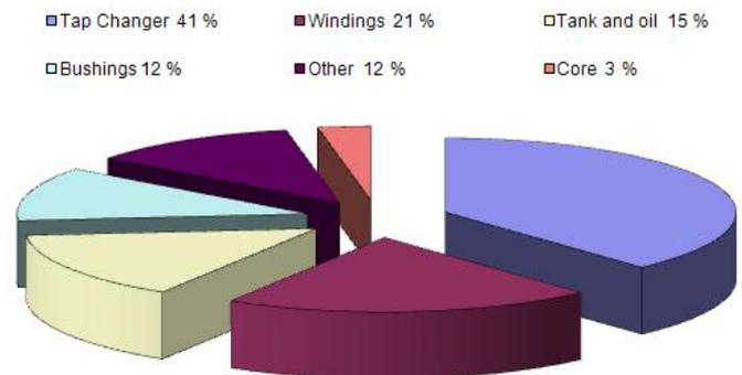
Fig.1. Allocation of failures through the parts of power transformers with the OLTC
