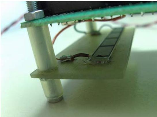
Fig 3. Segmented thermistor mounted on the auxiliary board
