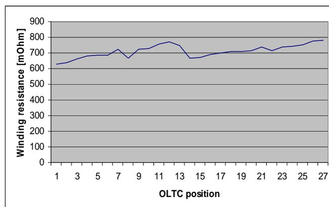
Fig.9. Static resistance measurement on T2
