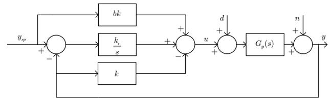
Fig.1. Plant  $G_p(s)$  with PI controller
