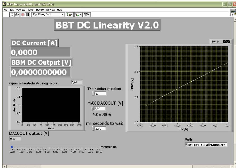
Fig.7. Front panel of program destined for linearity measurement of current sensors
