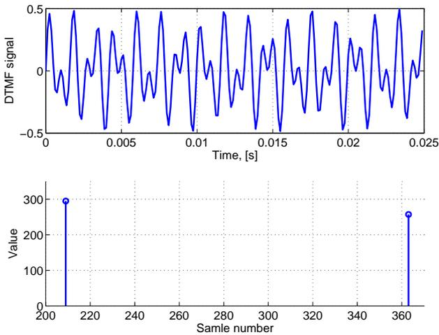
Fig.7. DTMF signal at the Goertzel cell input (above) and DTMF signal frequency spectrum (below).
