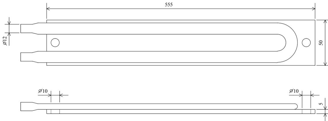
Fig.6. Shape and dimensions of the cooler
