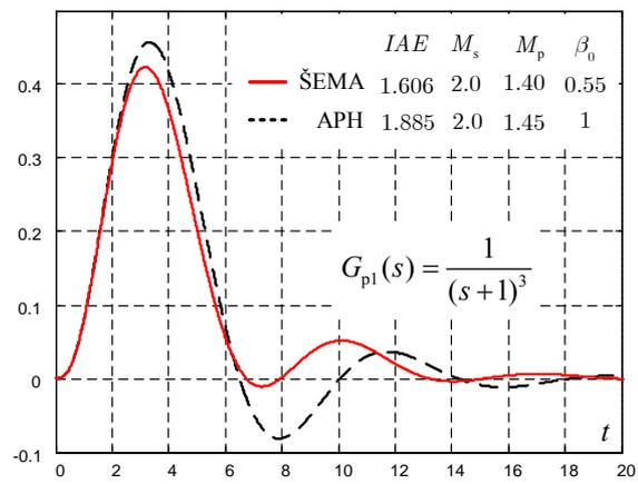
Fig.3. Load disturbance response for  $G_{p1}(s)$
