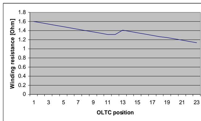
Fig.8. Static resistance measurement on T1
