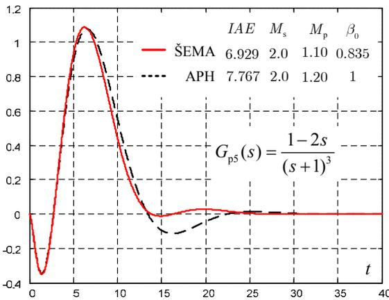
Fig. 7. Load disturbance response for  $G_{p5}(s)$
