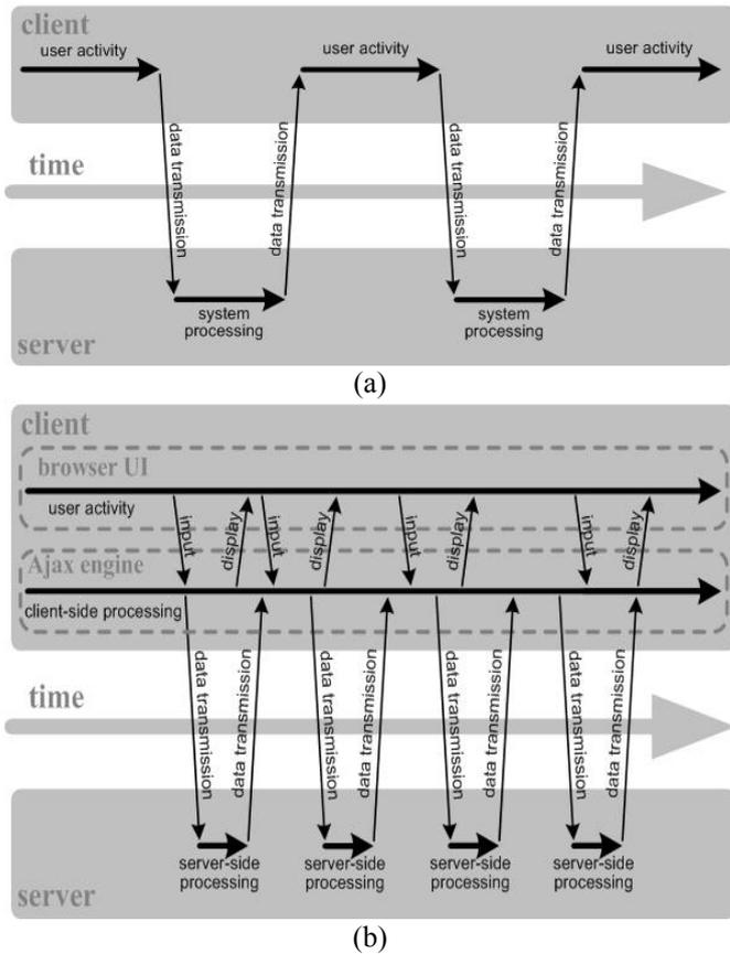
Fig.2. The synchronous interaction pattern of a traditional web application (a) compared with the asynchronous pattern of an AJAX application (b).
