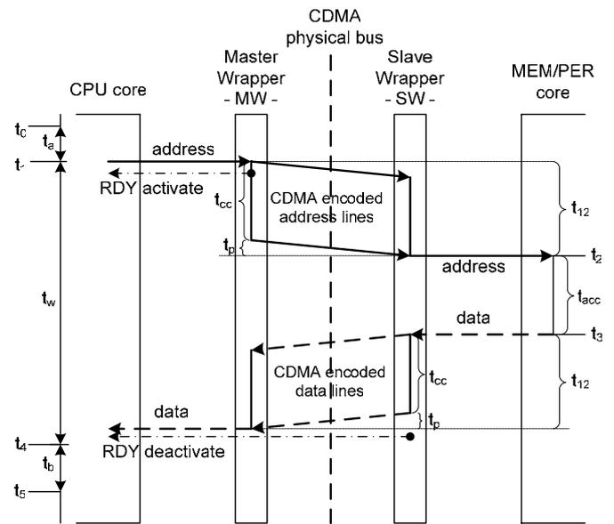
Fig.5. Signaling scenario of a Read processor cycle
