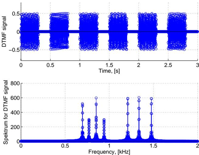
Fig.1. DTMF signal (Encoded tones), time signal (above) and frequency spectrum (below).
