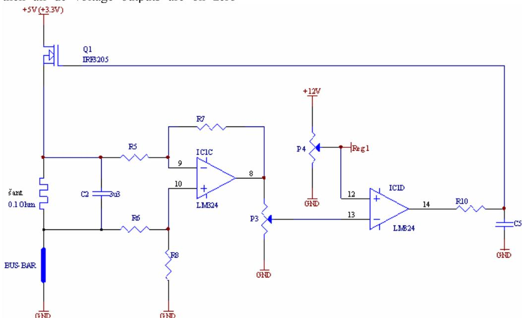
Fig.3. The basic configuration of the current regulator of one module
