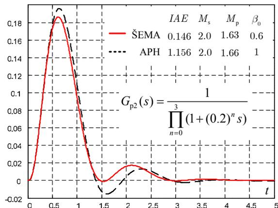
Fig.4. Load disturbance response for  $G_{p2}(s)$
