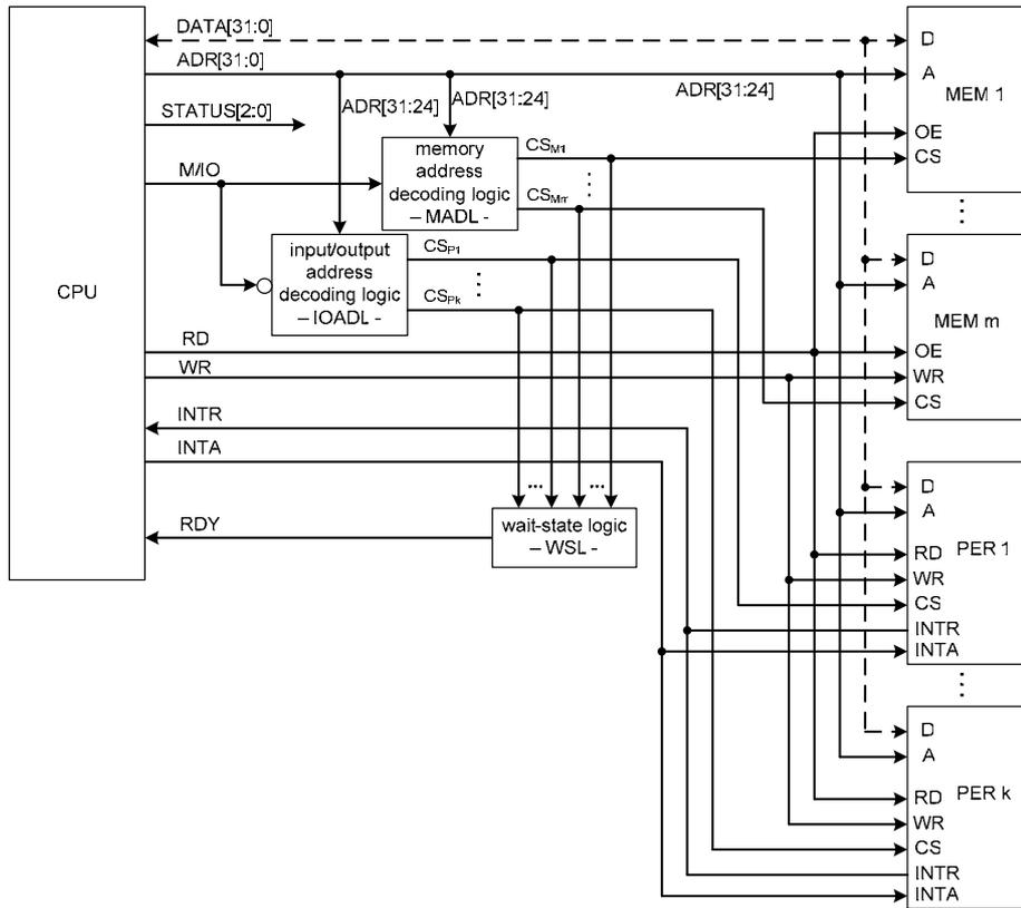
Fig.2. Uni-processor 32-bit system based on standard bus architecture
