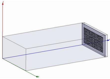
Fig.7. The simulation model of the high-impedance surface with the third order Hilbert curve inclusion
