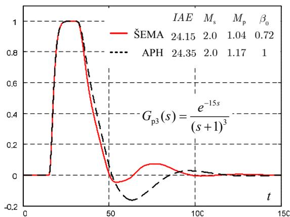
Fig.5. Load disturbance response for  $G_{p3}(s)$
