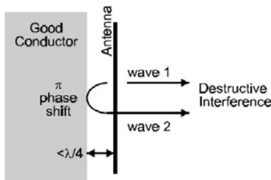
Fig.1. Destructive interference of reflected and emitted waves
