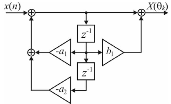
Fig.6. Second order Goertzel cell:  $a_1 = -2 \cos(2\pi f_i / F_s)$ ,  $a_2 = 1$ ,  $b_1 = e^{-2\pi f_i / F_s}$ .
