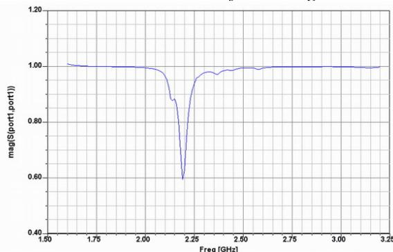
Fig.12. Magnitude of the refl. coeff. when there is no distance between the substrate and the end of the waveguide
