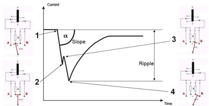
Fig.6. Dynamic behavior of the diverter switch
