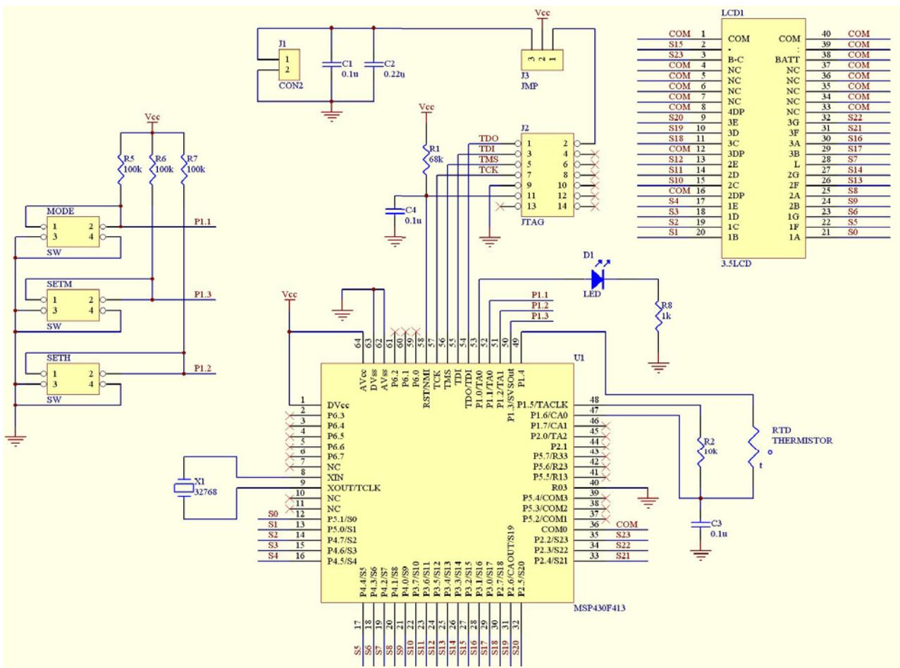
Fig.7. Realized thermostat's electric circuit schematic
