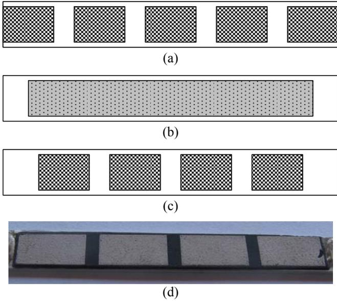
Fig.1. Segmented thick-film NTC thermistor: (a) bottom electrode, (b) NTC layer, (c) top electrode, (d) segmented thermistor construction.
