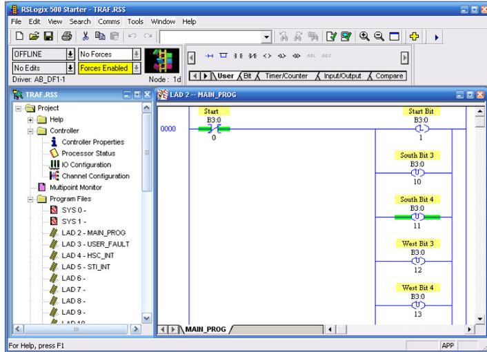
Fig.7. The main window of RSLogix 500 program
