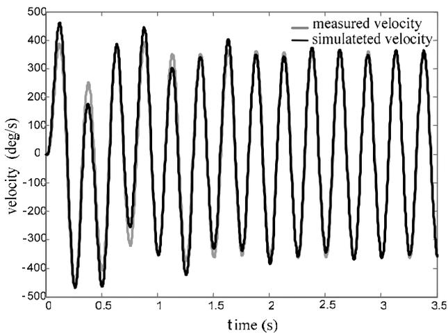
Fig.6. Measured and simulated apparatus speed
