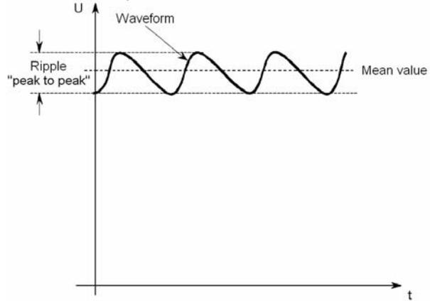
Fig.5. Ripple of output dc current
