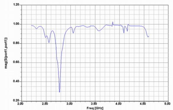
Fig.14. Simulated results of the structure with vias between the unit cells and the ground layer
