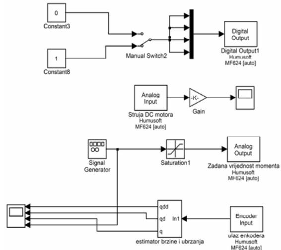
Fig.4. RTWTGT environment for data acquisition from the apparatus
