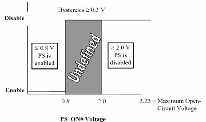
Fig.2. PS\_ON# signal characteristics
