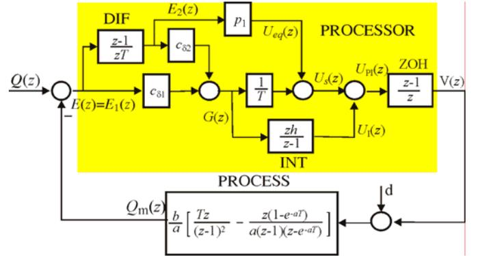
Fig.2. The closed-loop system structure,  $p_1 = \mathbf{c}_\delta^T \mathbf{A}_\delta$ .
