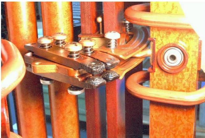
Fig.4. Damaged tap selector contacts
