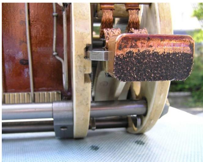
Fig.7. Aged contacts of the diverter switch
