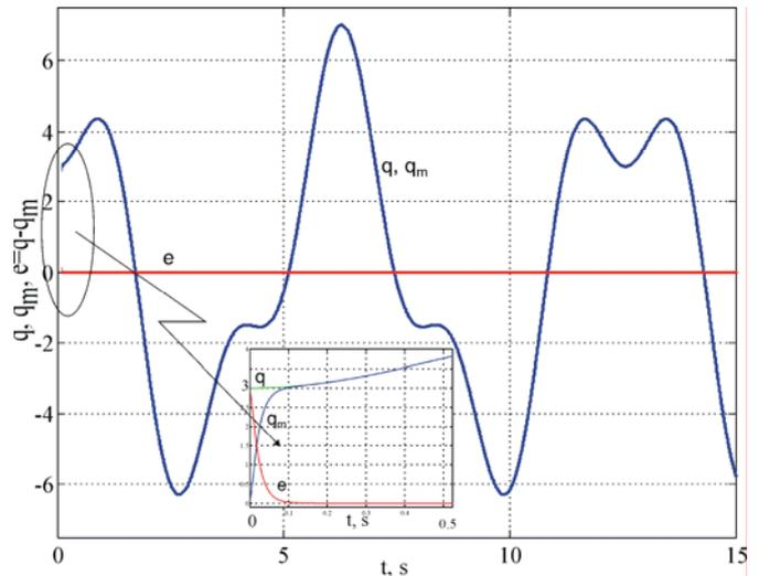
Fig.3. The response of the  $KG_m$  subsystem to reference  $q$ , (34), with integral action parameter  $h=1000$ .
