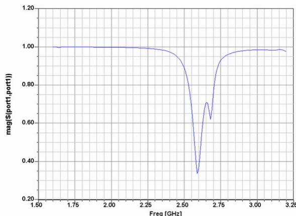
Fig.11. Magnitude of the refl. coeff. in case the separation between the substrate and the end of the waveguide is 2 mm
