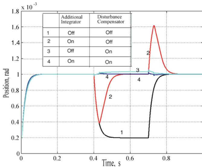
Fig.4. Step response of the proposed positional system for different conditions. Integral gain  $h$ : in the main controller (C)  $h=100$ ; in the controller  $K$  within the disturbance estimator  $h=1000$ .
