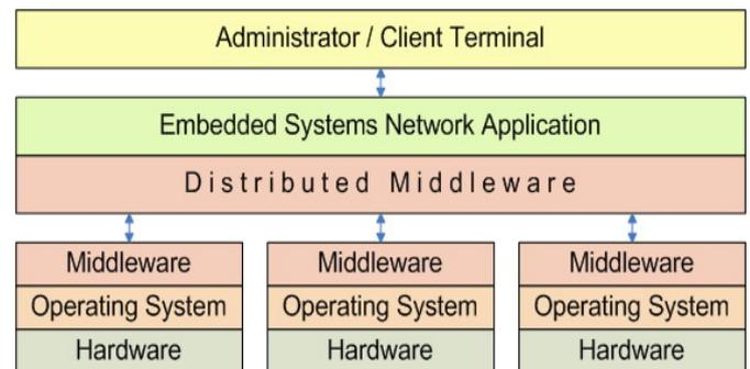
Fig.1. *Embedded systems network logical structure.*
