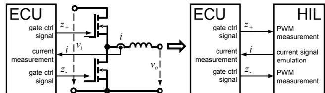
Fig. 1. Real system (left) and HIL simulation (right).
