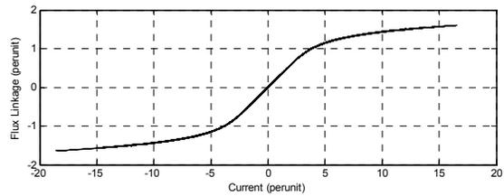
Fig. 3. Flux-current characteristic of the transformer core.
