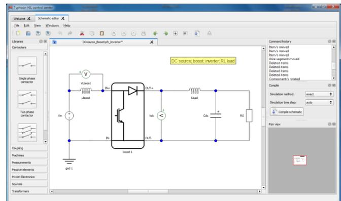
Fig. 2. Schematic editor view of the boost-converter circuit.
