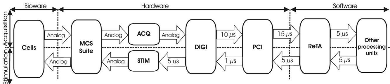
Fig. 7. Data propagation delays of the complete Hynet closed-loop. The minimum closed-loop processing period is  $46 \mu\text{s}$ . For our specification (10 kHz sampling frequency), more than  $50 \mu\text{s}$  are then available for the software during each period to close the loop.
