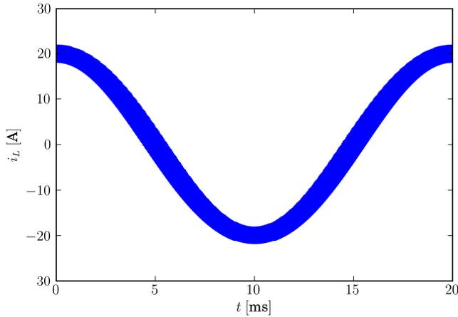
Fig. 10. Simulation, waveform of  $i_L$ , full period.
