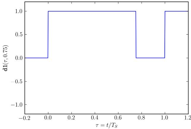
Fig. 7. Definition of the  $dl(\tau, d)$  switching function.
