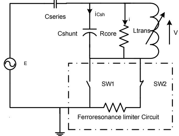
Fig. 5. (a) System equivalent circuit when ferroresonance suppression circuit is connected.
