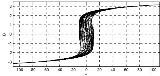
Fig. 4. Hysteresis loop of the transformer core.
