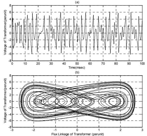
Fig. 7. Chaotic ferroresonance oscillation a) Time domain simulation b) Phase plane diagram.
