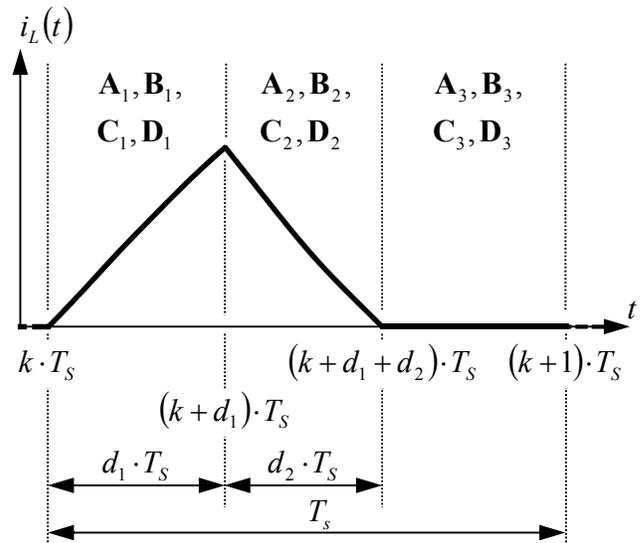
Fig. 6. Segmentation of the switching period  $T_s$ .
