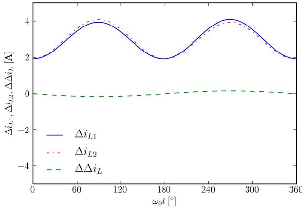
Fig. 4. Amplitude of the inductor current ripple.
