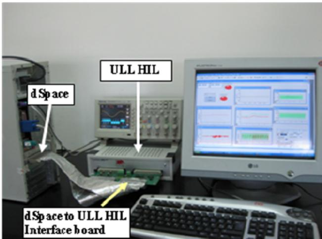
Fig. 11. CPS based on HIL and dSpace.
