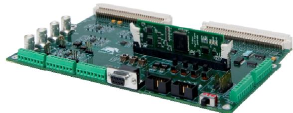
Fig. 9. HIL Docking Station for TI DSP.
