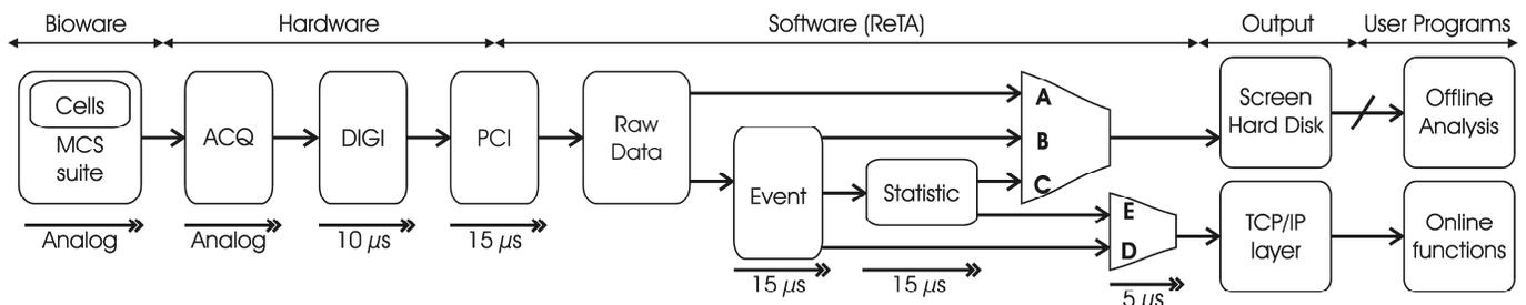
Fig. 5. Data propagation delays of the acquisition chain as described in Fig. 2 for different experimental configurations (A to E). The simplest experiment’s delay is 25  $\mu$ s for real-time raw data storage and monitoring (A). The most complex analysis requires 60  $\mu$ s (E).
