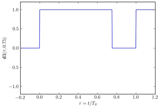
Fig. 7. Definition of the  $dl(\tau, d)$  switching function.
