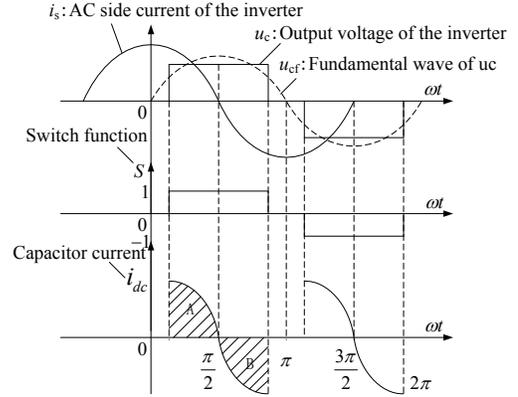
Fig. 4. Energy balance principle of the inverter bridge.
