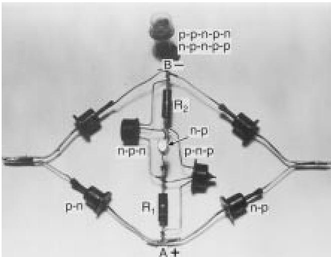
Fig. 9. Circuit model of a p-n-p-n switch [23].
