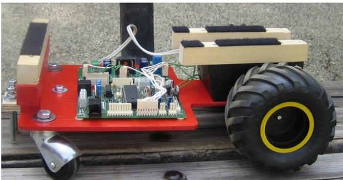
Fig. 3. Participant vehicle: structure, converter and control PCB.
