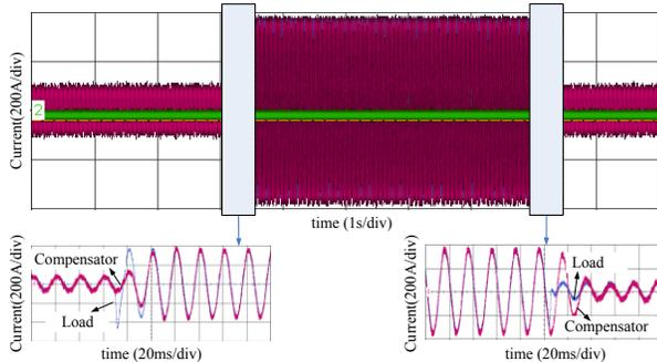
Fig. 14. Performance test for reactive compensation.
