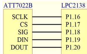
Fig. 4. Schematic diagram of the interface circuit between ATT7022B and LPC2138.
