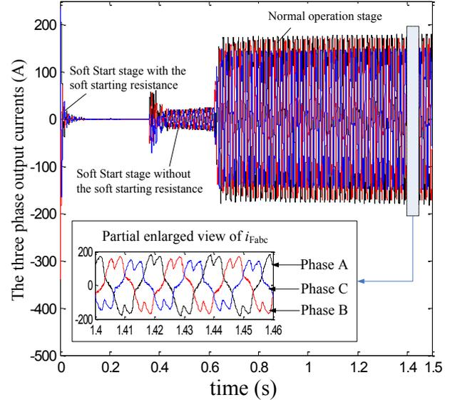
Fig. 7. Waveforms of three-phase output currents.
