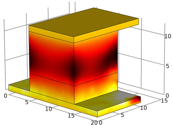
Fig. 1. Joule heating phenomena in memristor is demonstrated by thermal plot. The maximum joule heating problem in memristor can be clearly seen. It is due to the fact that when oxygen vacancies drift with mobility  $\mu_v$  throughout length  $D$  of memristor, it generates heat in the undoped area.
