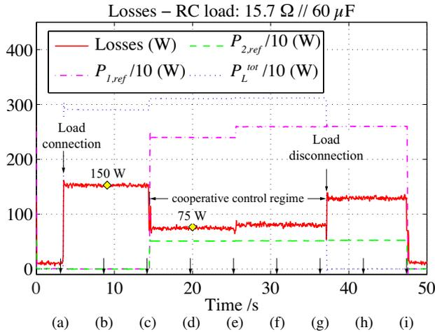
Fig. 12. Measured power losses for the experimental test.
