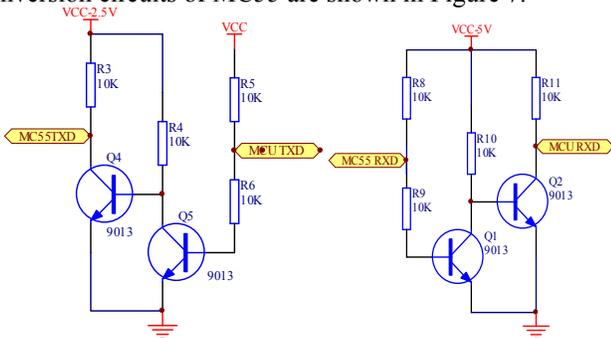
Fig. 7. Diagram of electric level conversion circuits.
