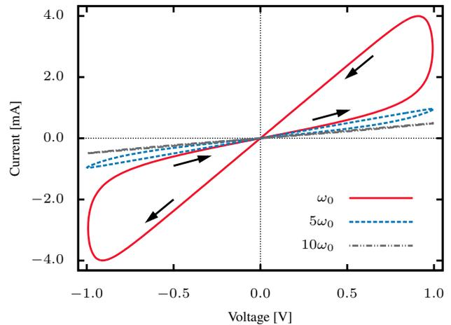
Fig. 2. Hysteresis loop of linear-ion drift memristor for frequencies:  $\omega_0$ ,  $5\omega_0$  and  $10\omega_0$  under the applied voltage bias of 1.0 V. The maximum current flows through the memristor at  $\omega_0$  is 4.0 mA
