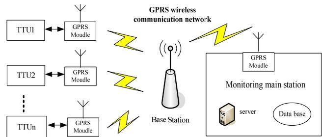
Fig. 1. The structure of transformer monitoring system.
