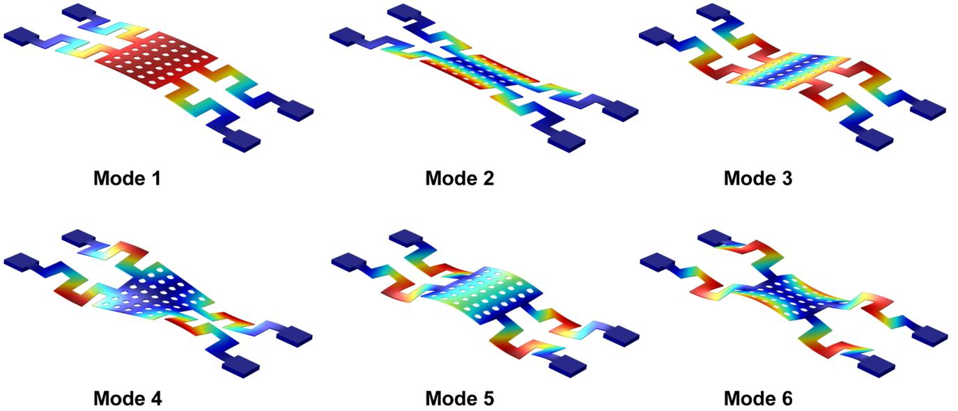
Fig. 7. First six modes with deformation of Au membrane is demonstrated that results from Eigenfrequency analysis in multiphysics environment.
