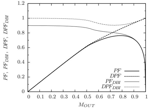
Fig. 8. Dependence of power factors and displacement power factors on the output voltage.
