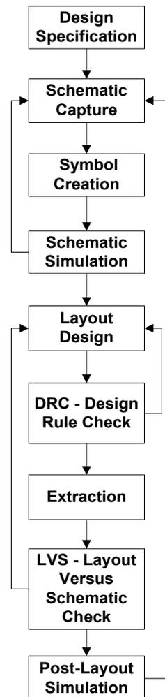
Fig. 3. Integrated circuit design flow in Cadence IC.
