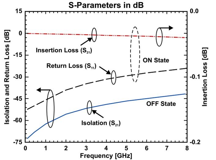
Fig. 8. RF performance measurements using the computation of  $S$ -parameters for the membrane shown in Fig. 4 results in isolation of 58 dB in OFF state of switch, insertion loss of 0.012 dB and return loss of 43 dB in ON state at 2 GHz.
