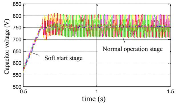
Fig. 13. Capacitor voltage of each power module (phase A).
