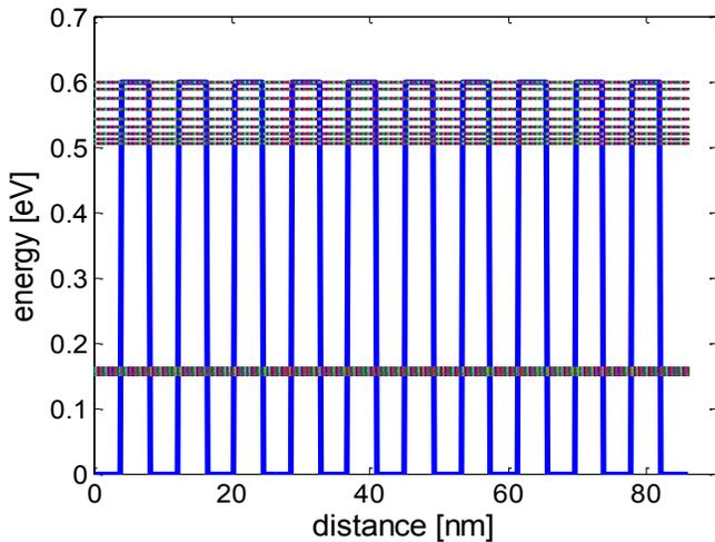
Fig. 4. Multiple-barrier case and formation of energy bands due to the interaction between the wells.
