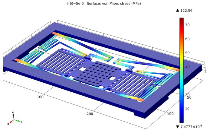
Fig. 4. Stress analysis in micro-membrane designed for RF-MEMS multipoint switch. The analysis is done using multiphysics environment with structural physics module. The simulation is shown demonstrating the deflection corresponds to force applied in vertical -Z-direction. The results shows that the maximum stress of 122.5 MPa on the edges of flexures for  $5 \mu\text{N}$  force applied.
