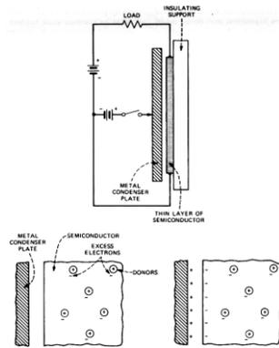
Fig. 1. Schematic of Shockley's field-effect idea [7].
