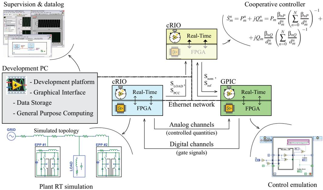
Fig. 8. Considered model for cooperative control test: real-time simulation system.
