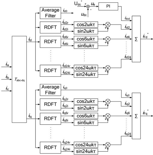
Fig. 1. Proposed reference current detection algorithm.
