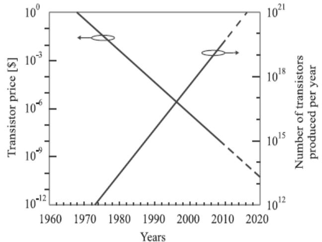
Fig. 14. Number of transistors produced per year and transistor price as a function of time [31].
