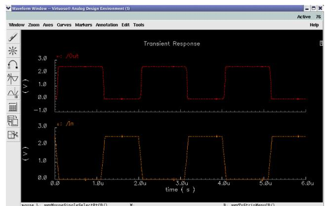
Fig. 7. Results of CMOS Inverter transient analyses.
