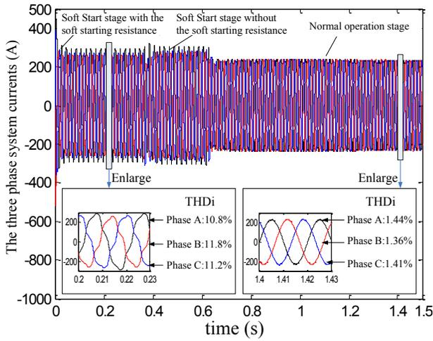
Fig. 10. Waveforms of three-phase system currents.
