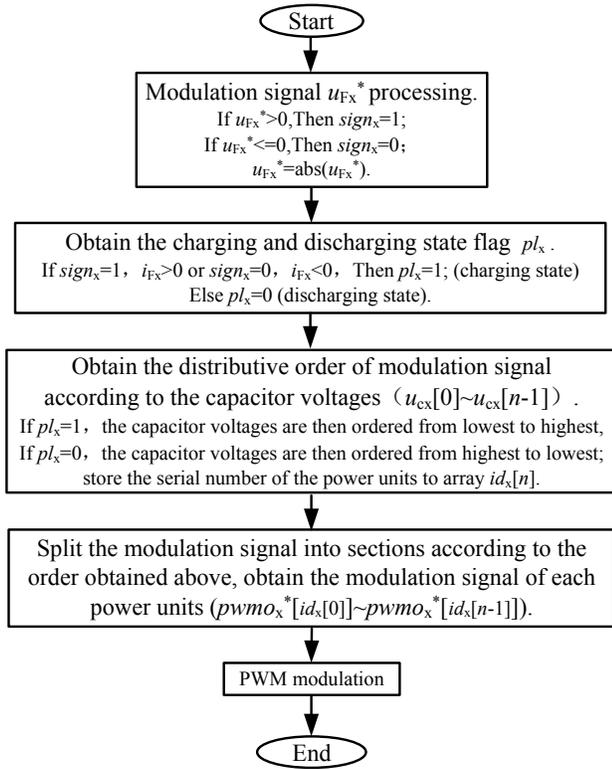
Fig. 5. Flow diagram of proposed individual balancing control strategy.
