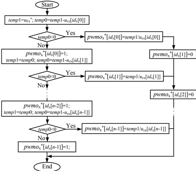
Fig. 6. Flow diagram of the modulation signal distribution process.
