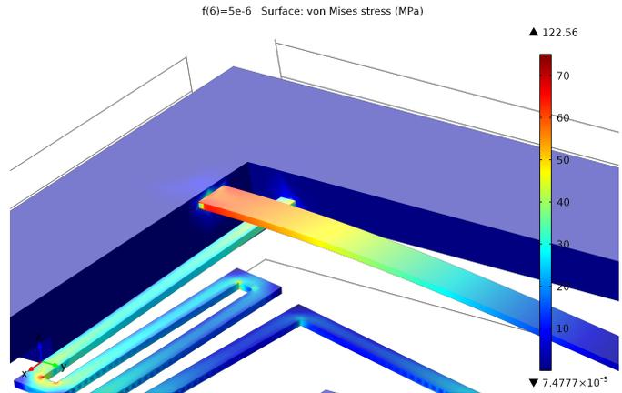
Fig. 5. Close-up view of stress prone area of Ti membrane. The flexures show maximum stress and thus the design can be further improved if required for different materials. The actual deformation is also shown in flexures.
