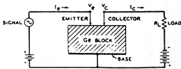
Fig. 2. Schematic of the "semiconductor triode" [8].
