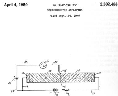
Fig. 4. Extract from the patent 2502488 (W. Shockley - Semiconductor Amplifier) [9].
