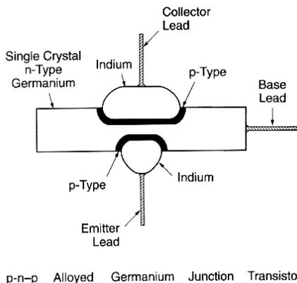
p-n-p Alloyed Germanium Junction Transistor
