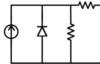
Fig. 4. Schematic circuit of a solar cell.
