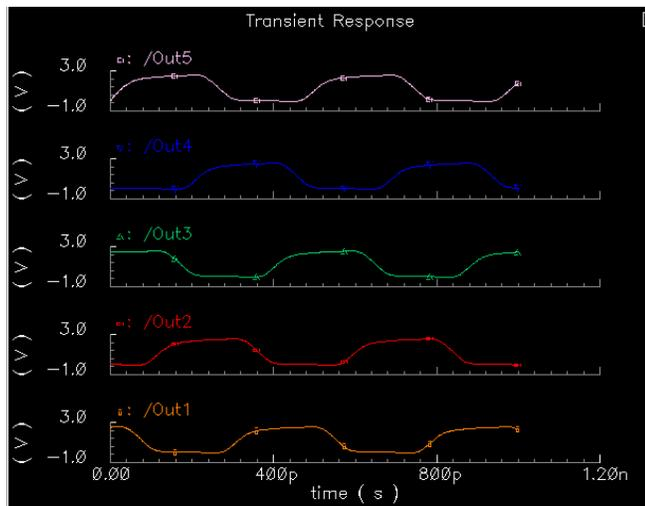
Fig. 12. Results of Ring oscillator transient analyses.
