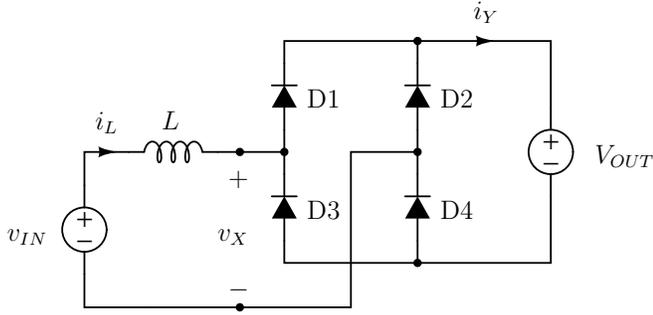
Fig. 2. Rectifier model applied in the analysis.
