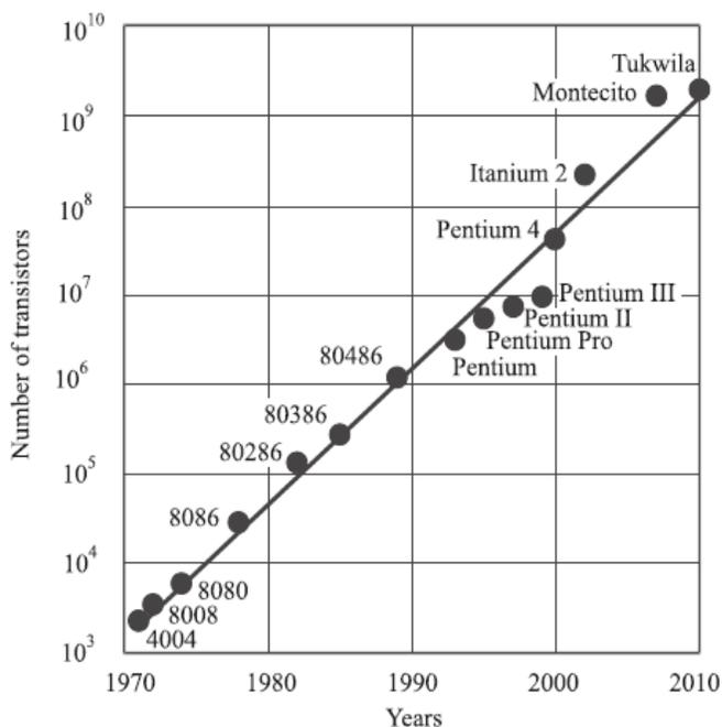
Fig. 12. Number of transistors in successive Intel processors as a function of time [29].
