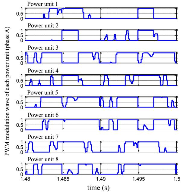
Fig. 12. PWM modulation wave for each power module.
