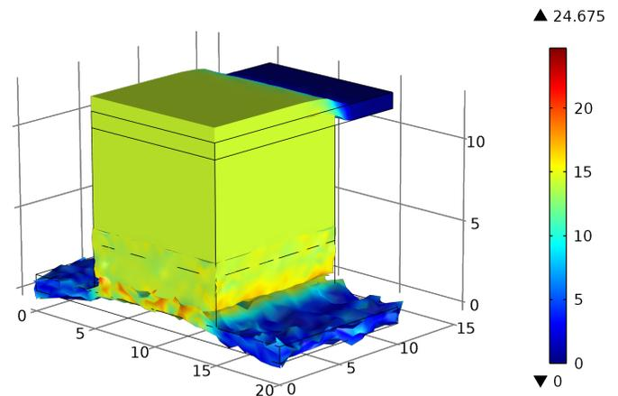
Fig. 3. Normalized current distribution in memristor due to the applied bias. The maximum current flows through the memristor is 24.675 A/m. Bottom deformed electrode is the positive electrode near doped region.
