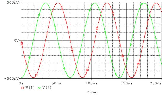
Fig. 9. Two quadrature voltage outputs at 15.92 MHz
