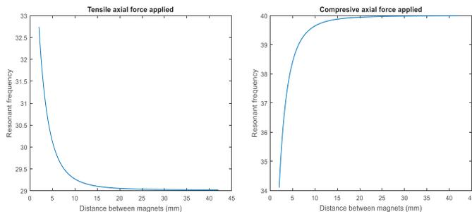
Fig.4. Resonant frequency vs. distance between tuning magnets
