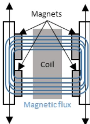
Fig.7. Coil-magnets configuration
