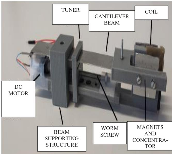
Fig.6. The prototype
