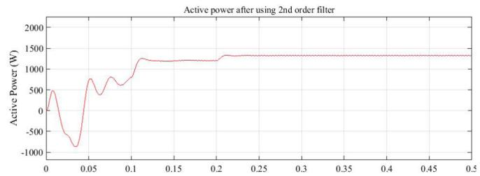
Fig. 9 The fundamental component of the active power of the three phases after using cascade 2<sup>nd</sup> order filters
