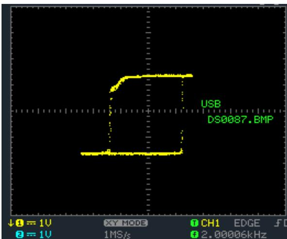
Fig. 13. Hysteresis phenomenon for the proposed Schmitt trigger.
