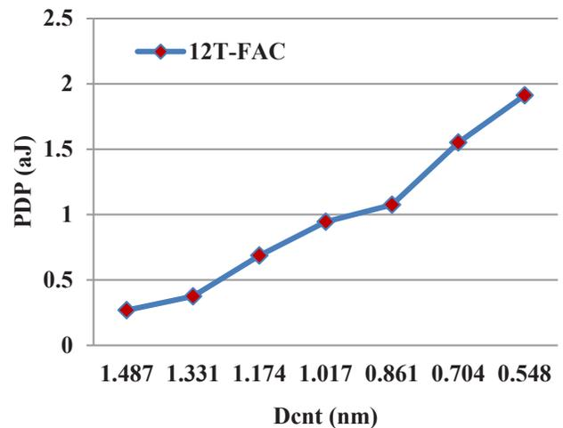
Fig. 7. PDP Versus Dcnt Variations for proposed circuit
