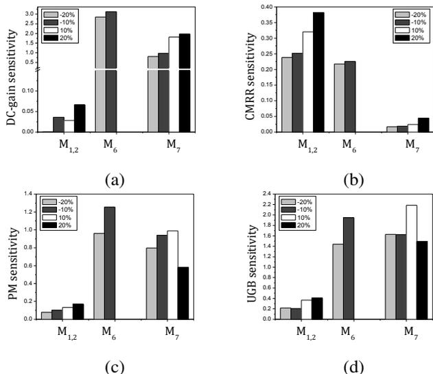
Fig. 5. Sensitivity of different parameters of the UTBSOI-opamp in the open-loop configuration with respect to tolerances of perturbation in the aspect ratio ( $W/L$ ) of  $M_{1,2}$ ,  $M_6$ , and  $M_7$  (a) DC gain, (b) CMRR, (c) PM, (d) UGB.
