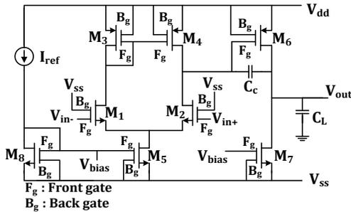
Fig. 2. Schematics showing the two-stage UTBSOI based opamp (UTBSOI-opamp).
