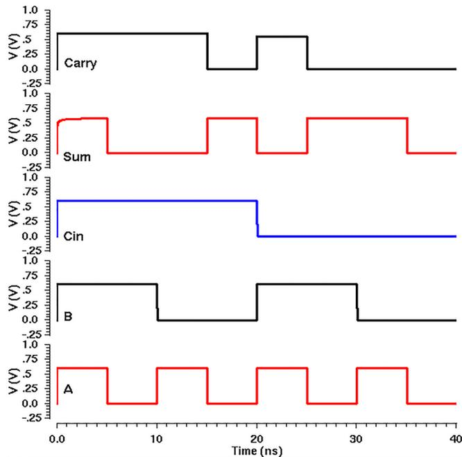
Fig. 6. Waveform of proposed 12T-FAC using CNFET
