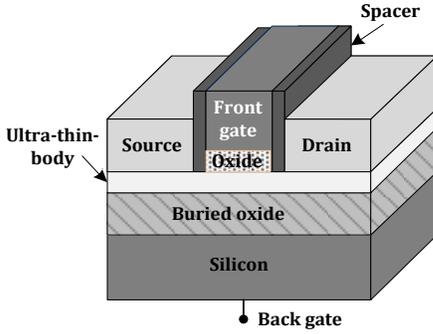
Fig. 3. Schematics showing 3D view of the UTBSOI transistor (Figure courtesy [14]).
