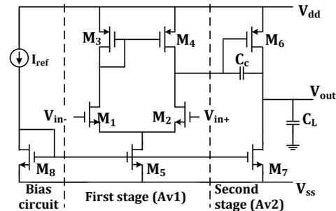
Fig. 1. Schematics showing the two-stage CMOS-opamp.
