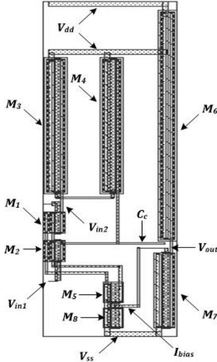
Fig. 4. Extracted layout view of the CMOS-opamp.
