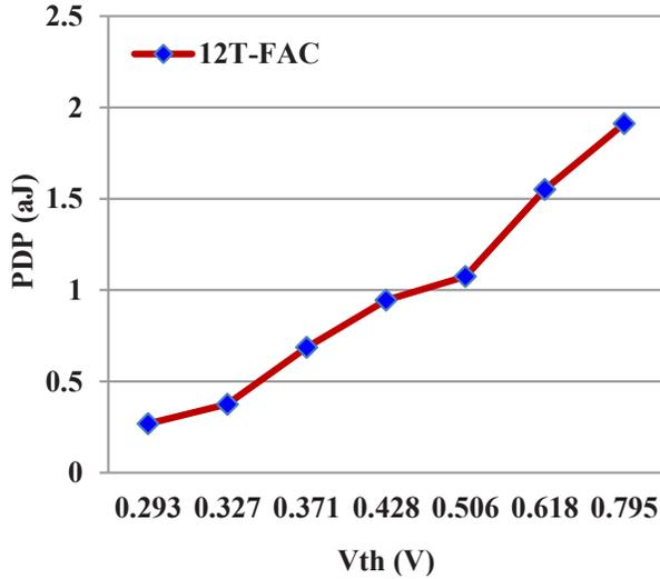
Fig. 8. PDP Versus Vth Variations for proposed circuit.
